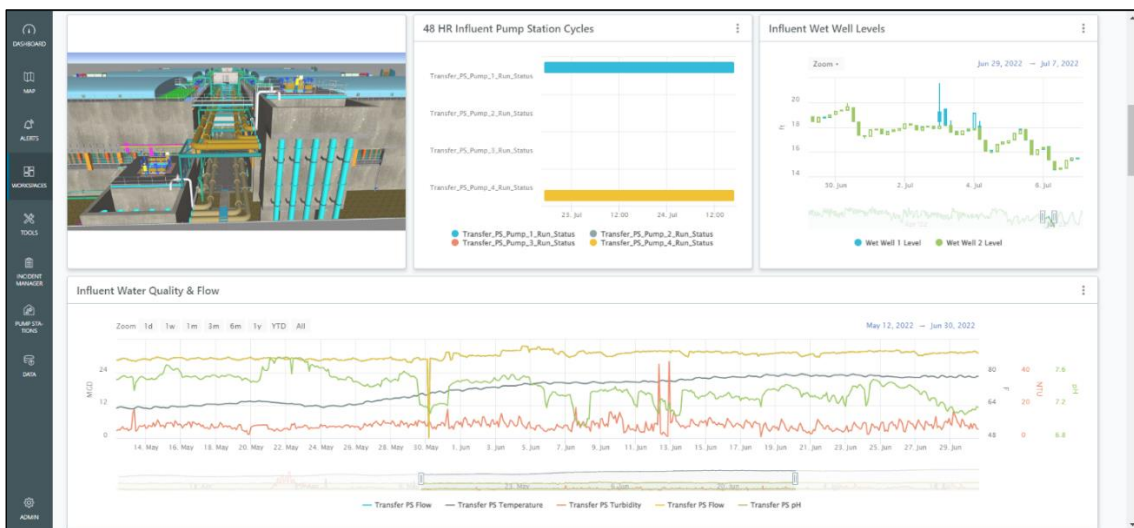
Figure 9 Analytics viewable within a user defined workspace for daily use that incorporates process flow diagrams, network maps, associated sensors and analytics, alert summaries, and data visualisation of live, forecast, and historical data.
